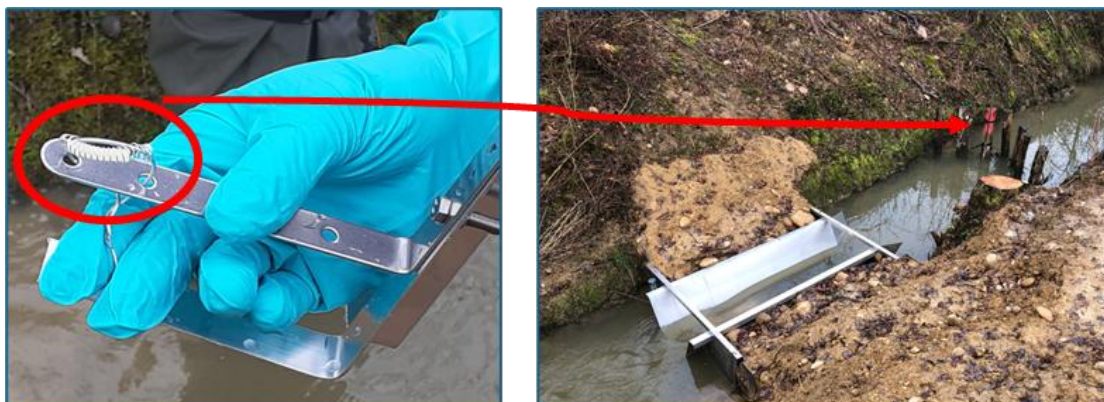
PACSiR rod attached to its hand-made support before being placed in a ditch equipped with a flow measurement flume
